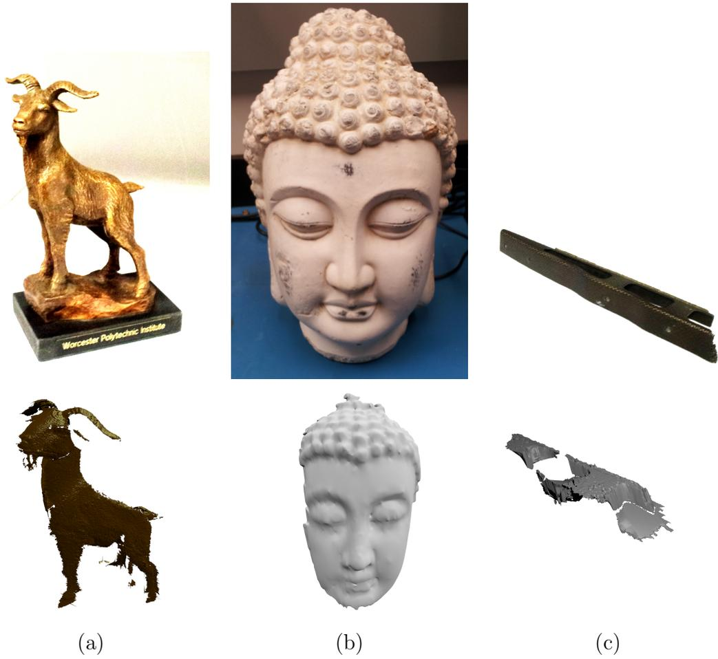
Figure 4.9: Sample meshes generated from *Pico Scan* and post-processed, along with photos of the objects from which they were generated. (a) WPI's "Proud Goat"; (b) a decorative statue; (c) a section of a broken component.
