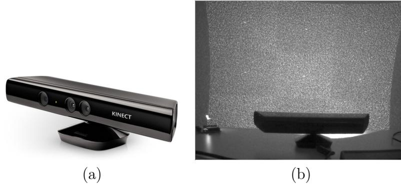
Figure 2.6: Microsoft Kinect. (a) the imaging device [Microsoft, 2012]; (b) projected pattern as seen through an infrared camera [Bernin, 2010].
